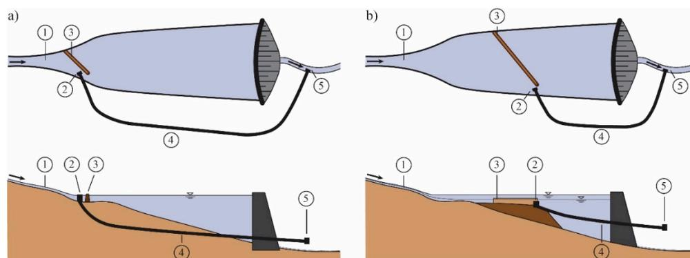
**Figure 1.** Illustration of two different types of SBT: (a) type A: free surface inflow at the reservoir head and (b) type B: pressurized inflow at the pivot point of the aggradation body downstream of the reservoir head; (1) reservoir head, (2) tunnel intake, (3) guiding structure, (4) SBT, (5) outlet structure (adapted from Müller-Hagmann, [48]).
