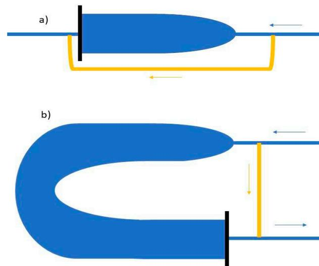
**Figure 4.** Sketches of two different sediment bypass tunnel configurations with type A intakes (Figure 1) with regard to reservoir shape and effects on SBT gradient. (a) Length of tunnel is nearly equal to the section it bypasses, and mean gradient of SBT is near equal to the river reach that has been impounded; (b) length of tunnel is shorter than the section it bypasses, and mean gradient of SBT is larger than the impounded river reach.
