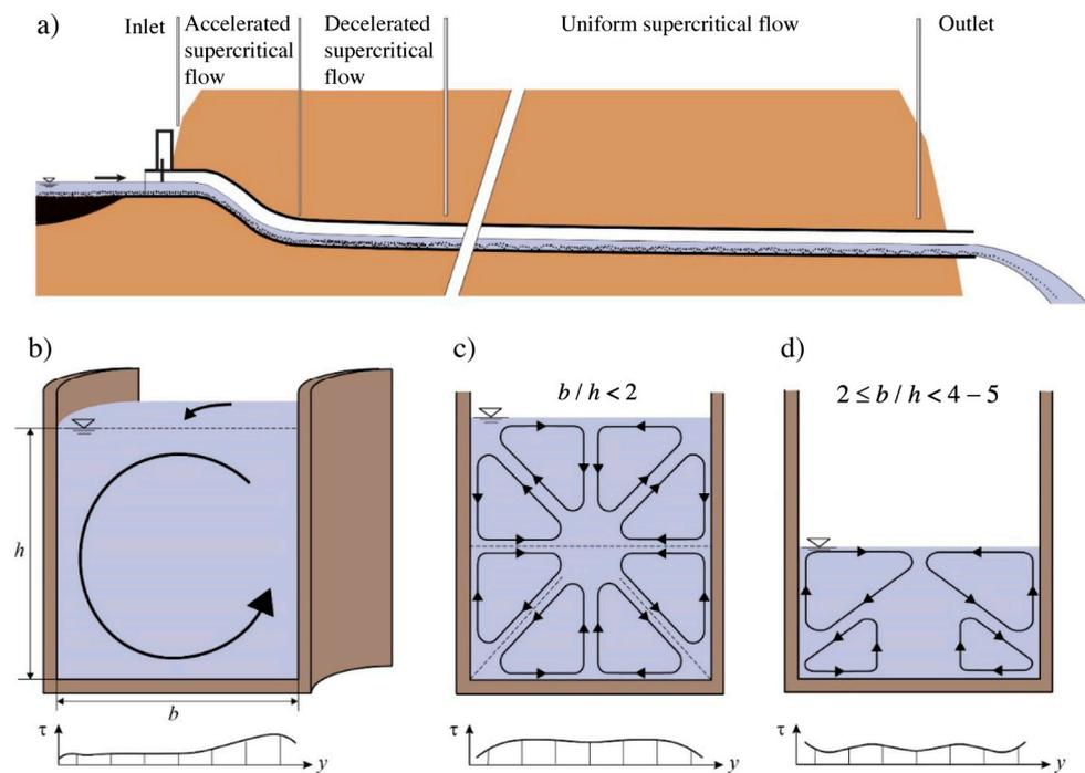
**Figure 2.** (a) Typical longitudinal section of SBT, and cross-section of SBT flow with Prandtl's secondary current of (b) first kind occurring at tunnel bends, and (c,d) second kind occurring in a straight tunnel section with (c)  $b/h < 2$  and (d)  $2 \leq b/h < 4$  to 5.
