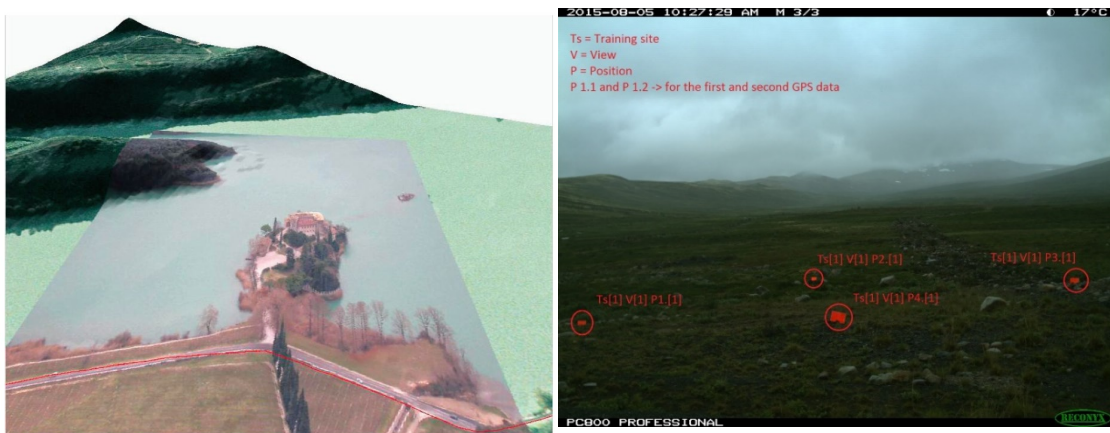
Figure 1: Orthorectification of oblique, tilted digital images. Left: the proof of concept by Neteler et al. (2005) Right: wildlife camera image with colour marked GCPs.
