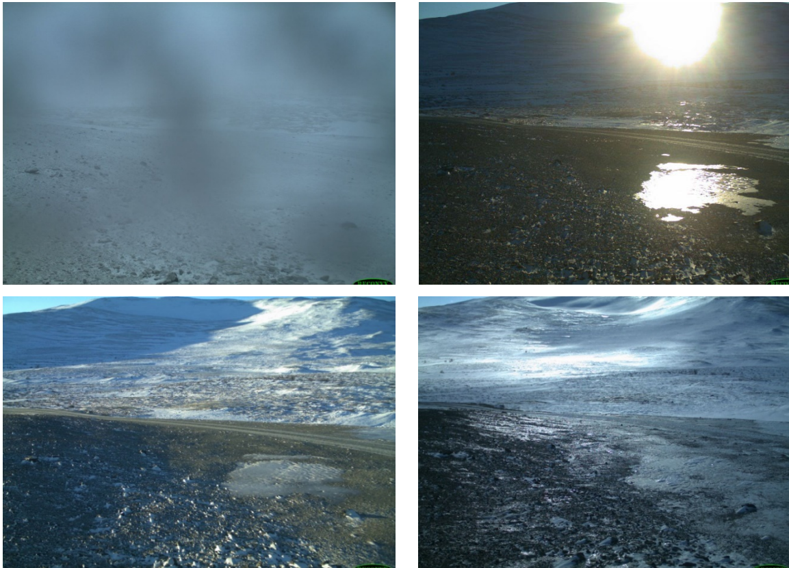
Figure 2: Examples of issues – Upper left: condensation, Upper right: sun shining into lens, Lower left: shadows and Lower right: reflection of sun on ice
