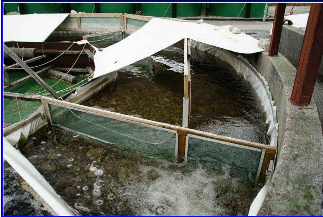
Fig. A5: One of the arenas during the 20 hours acclimatisation period seen from upstream. White tarps cover about 50% of each section. The "trap doors" are locked in place above the water surface and are ready to get dropped by removing the metal bolts that are attached to ropes.
