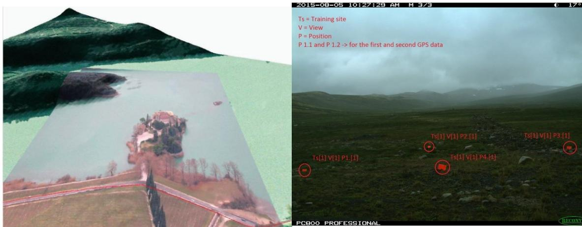
Figure 8: Orthorectification of oblique, tilted digital images. Left: the proof of concept by Neteler et al. (2005) Right: wildlife camera image with colour marked GCPs.
