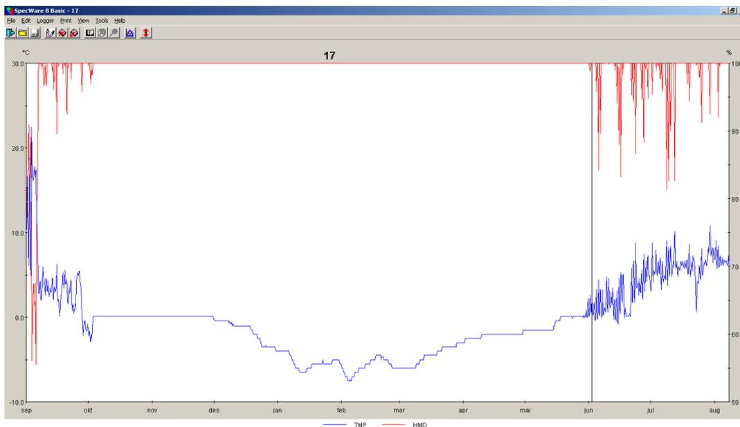
Figure 9: Data from temperature logger (in this case WatchDog B101 8K Temp Logger from Spectrum Technologies Inc.; <http://www.specmeters.com/weather-monitoring/data-loggers/b-series-loggers/b-series/>) can be used to identify snow cover and snow melt. The red line represents moisture, while the blue line is the temperature. The point where moisture and temperature begin to fluctuate indicates when the snow begins to melt.
