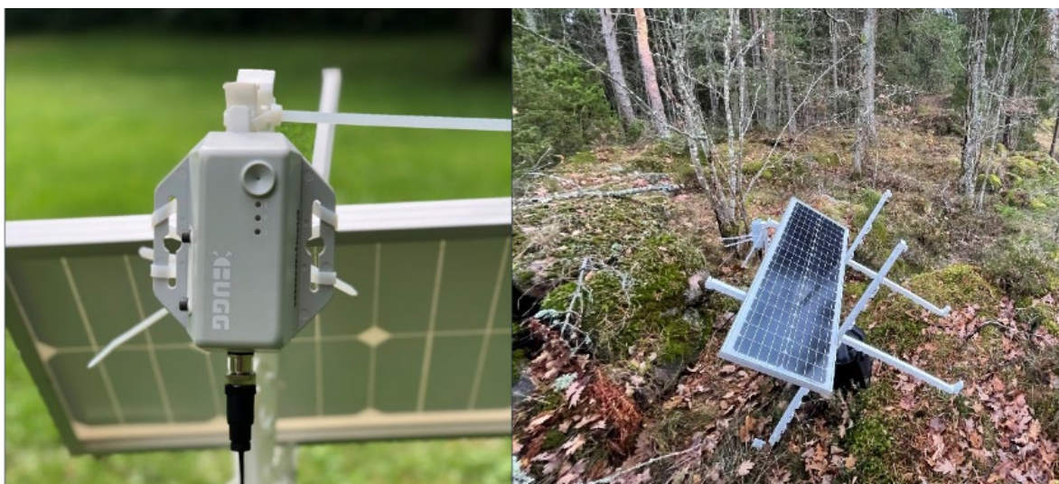
Figure 2: The Bugg recording devices and solar panels were mounted as illustrated at each of the 41 locations throughout Norway. The lithium battery and solar charge controller were placed on the ground nearby and sealed in a waterproof box (with an opening for cables in and out).
