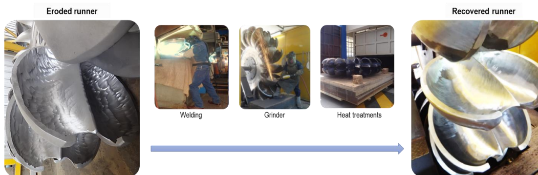
Figure 14. Main steps in the recuperation of the Pelton turbine by the welding process
