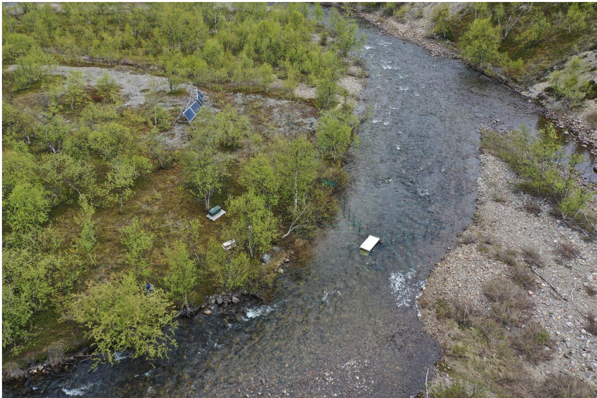
Figure 7. Simsonar FC stereo camera system installed to the River Gálldašjohka/Kalldasjoki. The white box in the middle of the river is the camera tunnel unit. Guiding fences goes from the tunnel unit downstream to both shores. Data recording and solar power systems are situated on the shore (left hand side). Photo: Mikko Kytökorpi.
