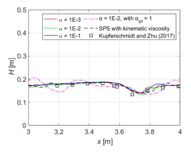
**Figure 5.** Centerline water-surface elevation along the selected section of HOR case for dp = 1.5 cm and various viscosity treatments.
