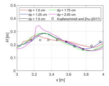
**Figure 4.** Centerline water-surface elevation along the selected section of VUS case for  $\alpha = 0.01$  and various *dp*.
