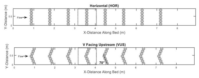
Figure 2. Plan view of the geometries used in the validation, taken from [45].
