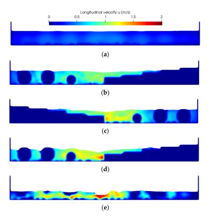
**Figure 12.** Longitudinal velocity *u* for the  $Q_2$  case, looking in the downstream direction, at crosssections. (a) x = 1.5 m (i.e., upstream of the first row of obstacles), (b) x = 3 m (i.e., first line of cylinders), (c) x = 6 m (i.e., second line of cylinders), (d) x = 9 m (i.e., third line of cylinders), and (e) x = 11 m (i.e., downstream of the last line of obstacles).
