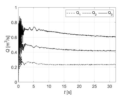
Figure 10. The different flow rates reached steady state condition after 30 s of simulation.
