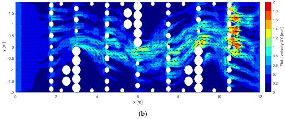
Figure 14. Velocities close to the bottom at z = 0.05 m plane for the  $Q_2$  case (a) with smooth bed and (b) bed roughness.
