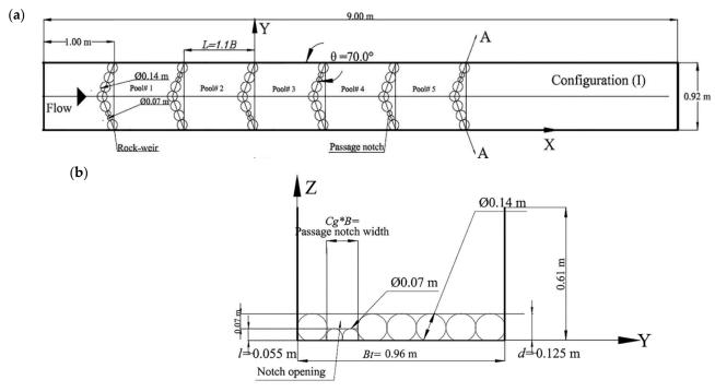
Figure 7. The model domain. (a) Plan view and (b) sectional A-A view—both taken from [16].
