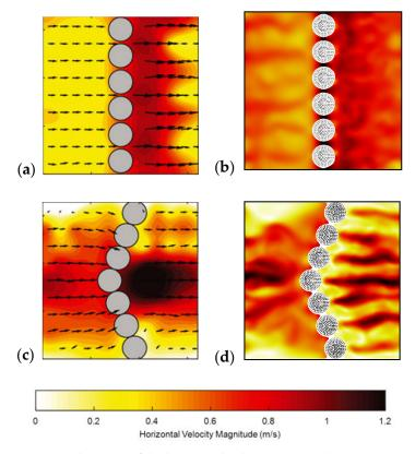
**Figure 6.** Plan view of the horizontal velocity magnitude at z = 0.08 m plane. (a) HOR experiment (b) HOR model, (c) VUS experiment, (d) VUS model. Dots in (b,d) represent solid particles of spheres. Figure 6a,c are taken from the reference study.
