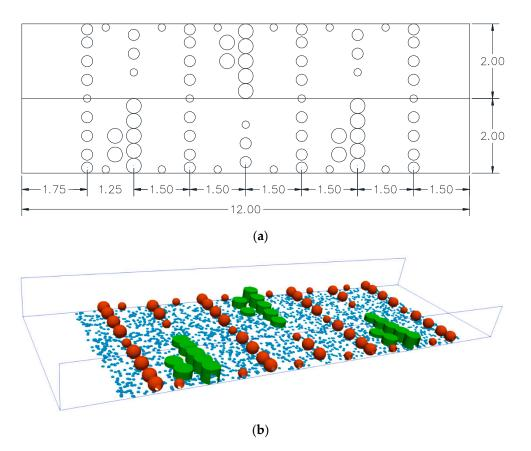
**Figure 9.** The model geometry (**a**) with a smooth bed (dimensions in meters) and (**b**) with bed roughness elements. Colors indicate bed roughness elements (blue), substrate spheres (red), and cylinders (green). Flow from left to right.
