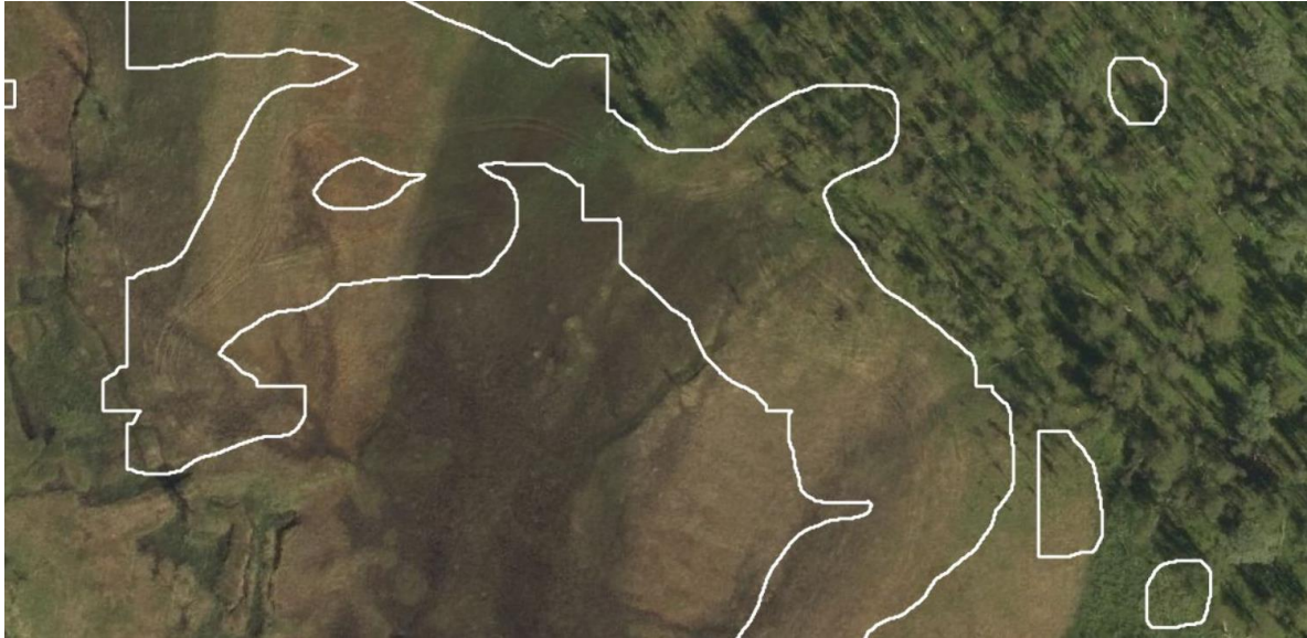
Figure 21. Example of areas where wheel rut detection works quite well even in aerial images
