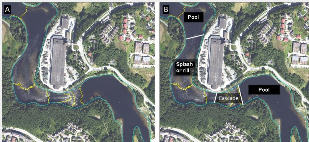
Figure 24. Classification of part of the River Nidelva (123.Z) into mesohabitat units: (A) *Norge i bilder* image (2010); (B) mesohabitat classifications. Yellow contours show LiDAR-derived surface elevation (contours are at 0.5 m intervals).
