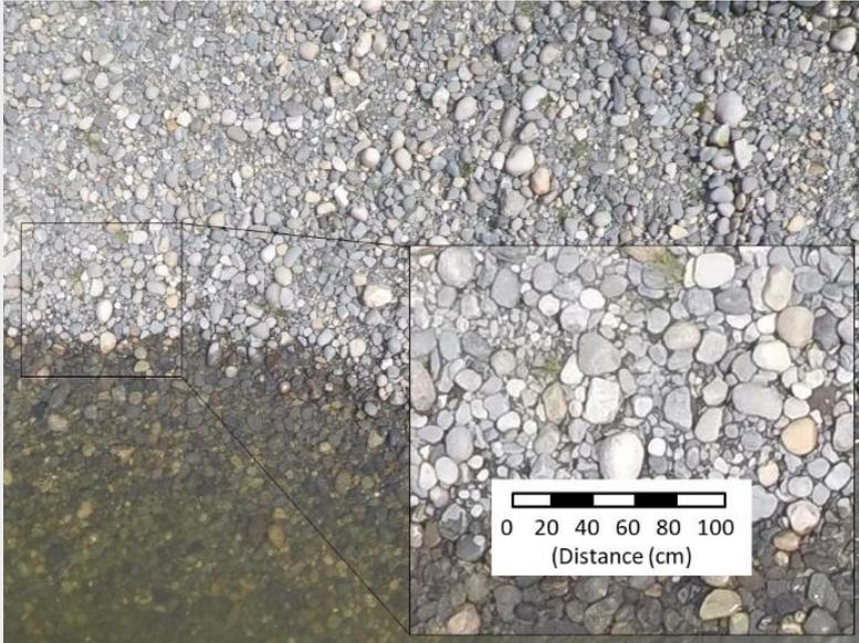
Figure 2. Example of UAV imagery obtained from a multi-rotor UAV operating at an elevation of less than 10 m (River Gaula, Vassdrag Nr: 122.Z). Pixel length is < 3 mm.
