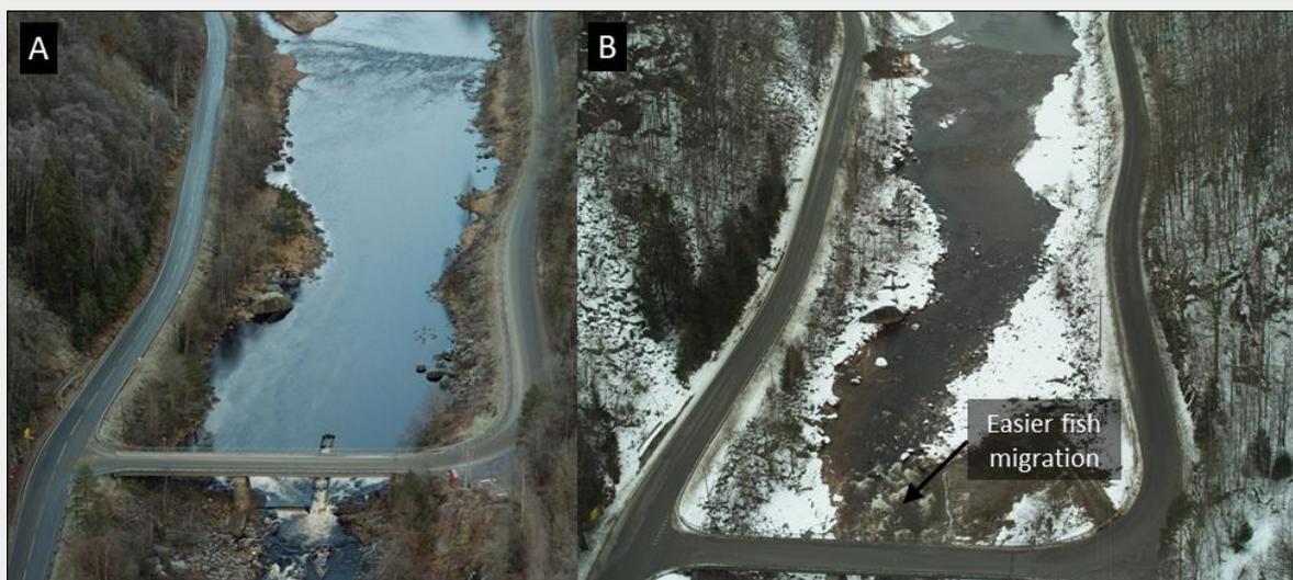
Figure 35. Oblique aerial photographs of the River Mandalselva (022.Z) obtained from a helicopter survey: (A) before removal of a weir; (B) after removal of a weir. See <https://brage.nina.no/nina-xmlui/bitstream/handle/11250/2657971/Forseth%20Mandalselva%202020.pdf?sequence=1&isAllowed=y>. Source: Tor Kviljo
