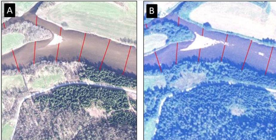
Figure 21. Surveys of wetted width of the River Nausta (084.7Z) using *Norge i bilder* images: (A) discharge =  $20.1 \text{ m}^3 \text{ s}^{-1}$ ; (B) discharge =  $5.2 \text{ m}^3 \text{ s}^{-1}$ .
