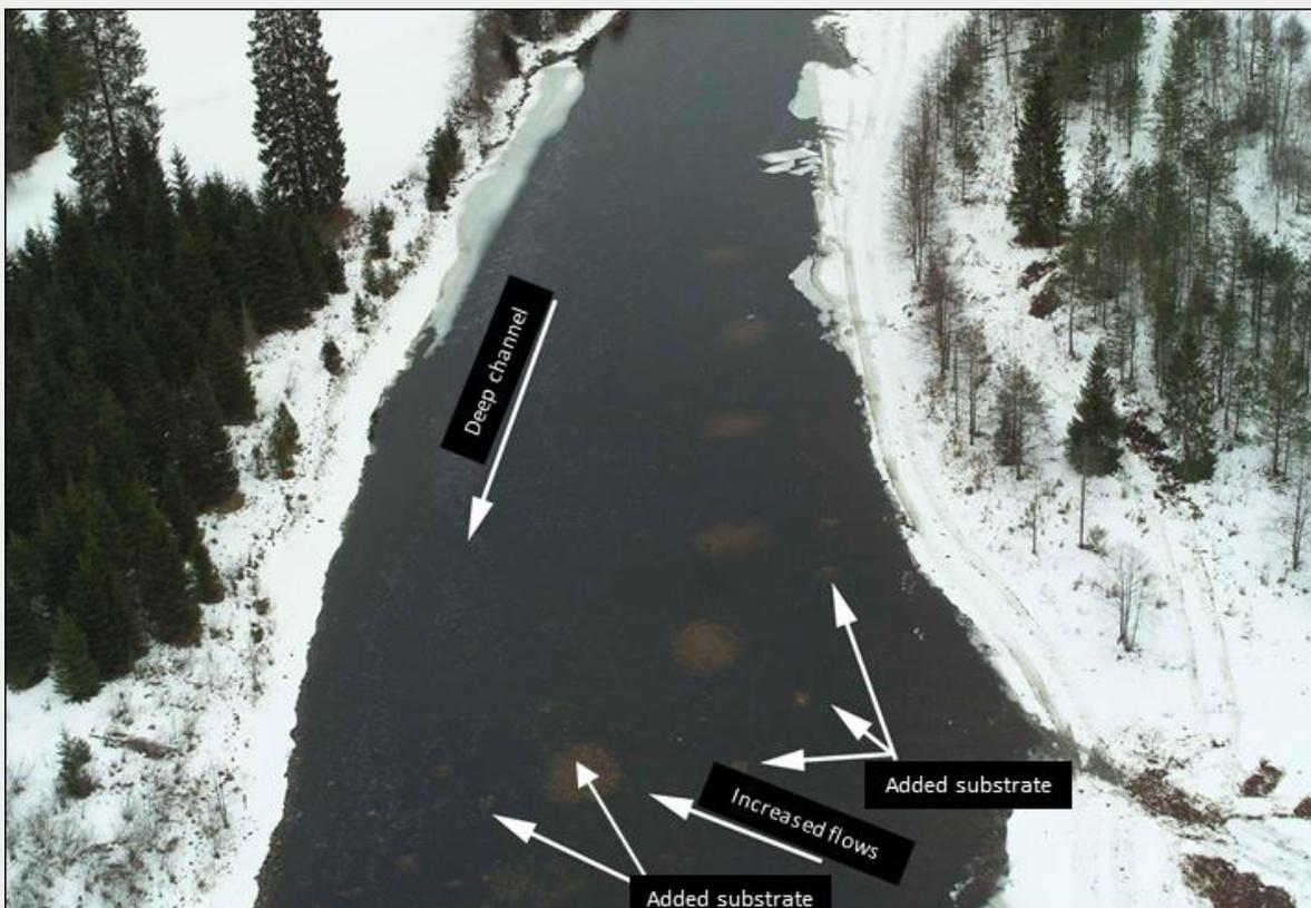
Figure 36. Oblique aerial photograph of the River Mandalselva (022.Z) obtained from a helicopter survey showing substrate additions and improved flow conditions. Source: Tor Kviljo.
