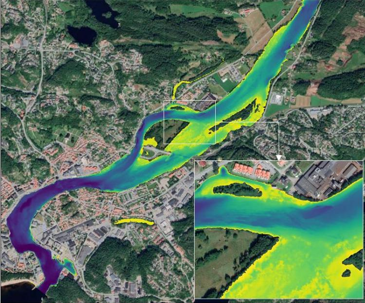
Supplementary figure 1. Bathymetric DEM as derived from a green LiDAR survey of the River Mandalselva (022.Z) near the outlet. The color scheme ranges from dark blue (< -17 masl) to yellow ( $\approx$  -2 masl).
