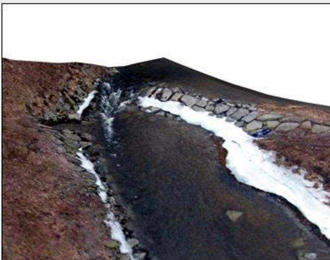
Figure 58. UAV image of the River Børsa (122.1Z) draped over a 1 × 1 m DSM. NB: the z-scale has 2× magnification.
