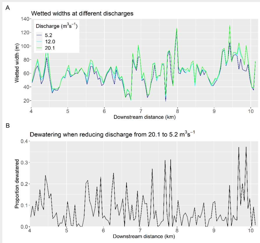
Figure 22. Cross-sectional profile of the River Nausta (084.7Z) as determined from *Norge i bilder* imagery: (A) discharge – wetted width relationships; (B) proportion dewatered at low discharge.
