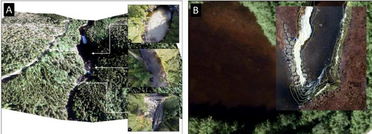
Figure 59. Integration of airborne surveys with GIS data: (A) Norge i bilder image of the River Nævre (123.4Z) draped over a DTM; (B) UAV and Norge i bilder images of the River Børssa (122.1Z). In (A), side panels show UAV images; in (B), contours are at elevation differences of 0.1 m.
