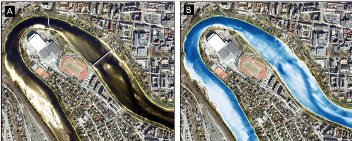
Figure 23. Lower watercourse of the River Nidelva (123.Z): (A) *Norge i bilder* image (2006); (B) predicted water column depth from a HEC-RAS simulation at a discharge of  $135 \text{ m}^3 \text{ s}^{-1}$  (Source: Ana Juarez, NTNU). In A, the area within the river confines (yellow polygon) has been contrast enhanced.
