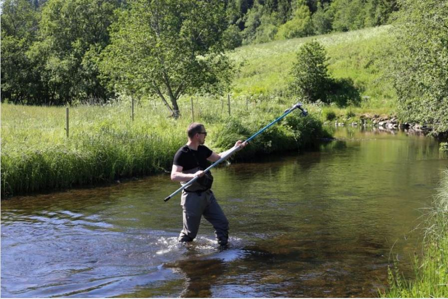
Figure 37. Photo surveying conducted by wading through the River Vigda (122.2Z) using a pole-mounted camera. Source: R. Hedger.
