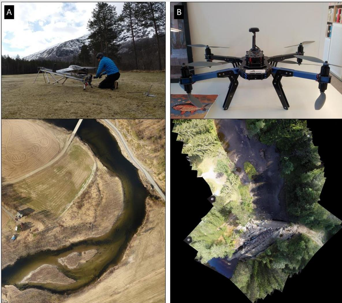
Figure 25. UAV types and associated imagery: (A) fixed-wing UAV, and (B) multi-rotor UAV. Photo source: A. Foldvik.
