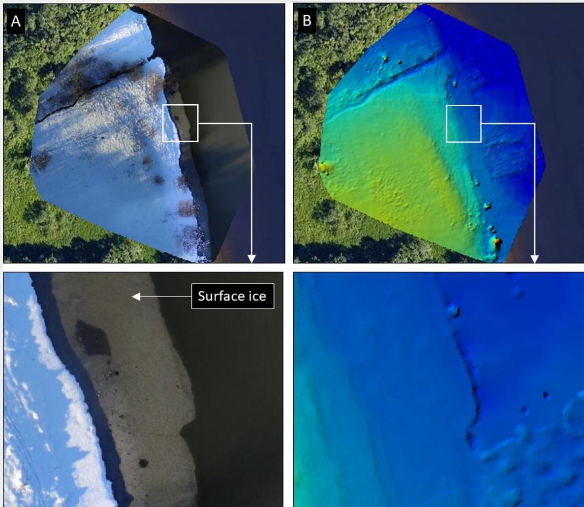
Figure 30. UAV survey of the River Nidelva (123.Z): (A) orthomosaic; (B) digital surface model (DSM) created through Structure from Motion (SfM).
