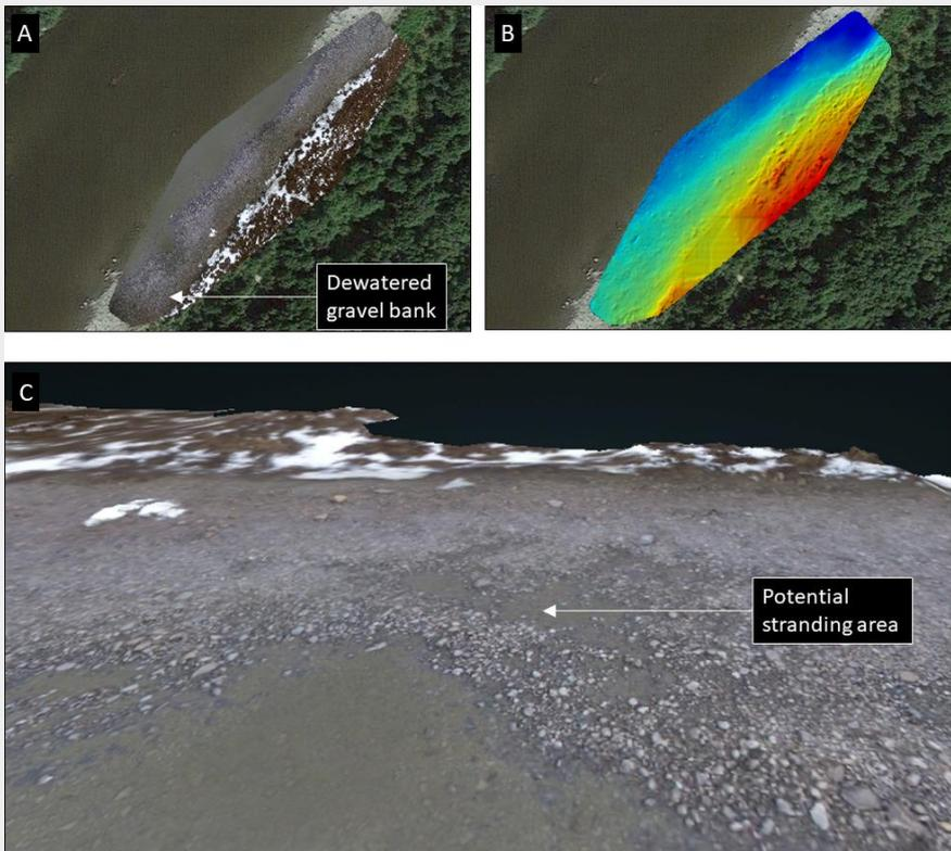
Figure 29. UAV survey of the River Gaula (122.Z): (A) orthomosaic; (B) digital surface model (DSM) created through structure from motion (SfM); (C) oblique view of draped surface.
