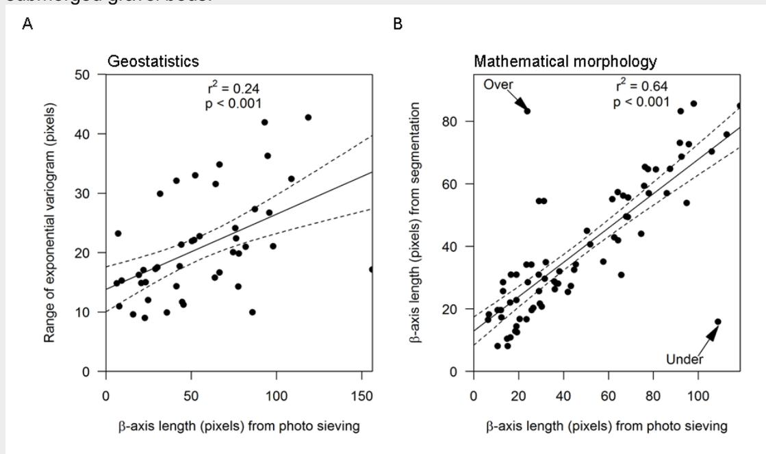
Figure 34. Comparison between estimated substrate size and manual measurement from imagery from photo sieving: (A) geostatistical approach; and (B) mathematical morphological approach.
