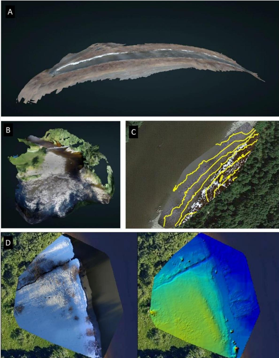
Figure 57. Examples of errors associated with SfM-based generation of DSMs: (A) distortion caused by camera barrel distortion in images without GPS-encoding; (B) distortion at the edges of the area imaged; (C) incorrect estimates of surface elevation across a dewatered/watered interface; (D) incorrect estimates of surface elevation from shadows. All DSMs were created in OpenDroneMap. In (C), yellow contour lines show elevations at 0.5 m intervals.
