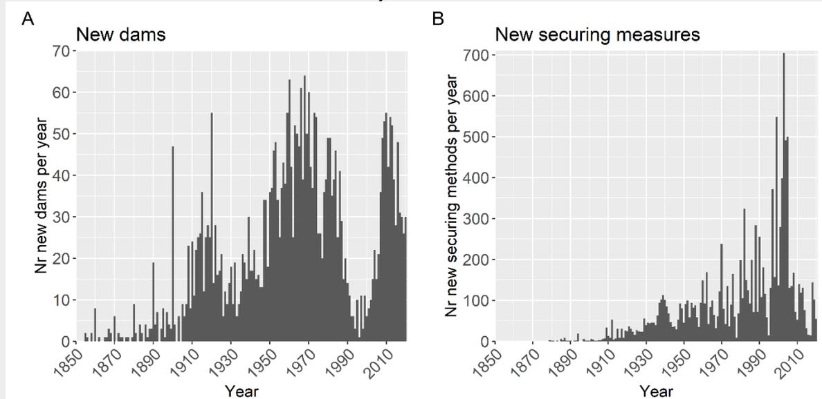
Figure 13. Infrastructure development in Norwegian watercourses: (A) dams; (B) securing measures. NB: Only dams or securing measures that have a registered construction date have been included.
