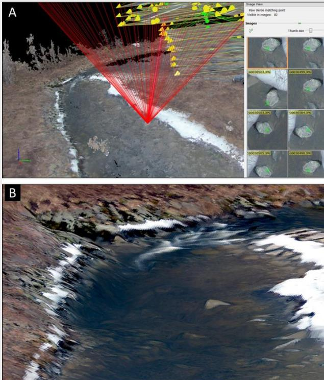
Figure 31. Structure from motion (SfM) depth extraction from UAV images of the River Børsa (122.1Z): (A) reconstructed image overlain on digital surface model (DSM) generated from multiple images; (B) zoomed-in area showing stretch immediately downstream of the weir.
