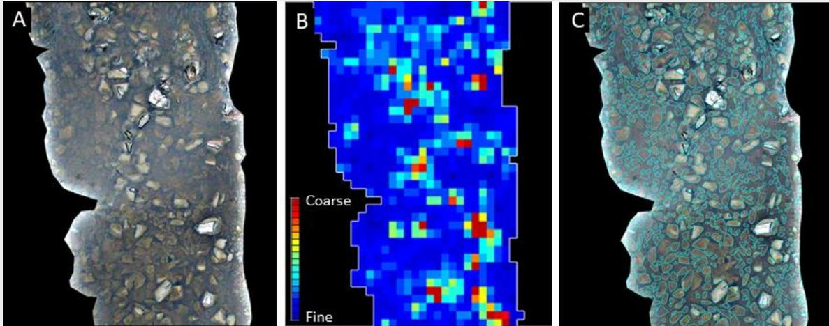
Figure 33. Texture-based classification of substrate size in a UAV image of the River Børsea (122.1Z): (A) original image; (B) geostatistical approach; (C) mathematical morphological approach.
