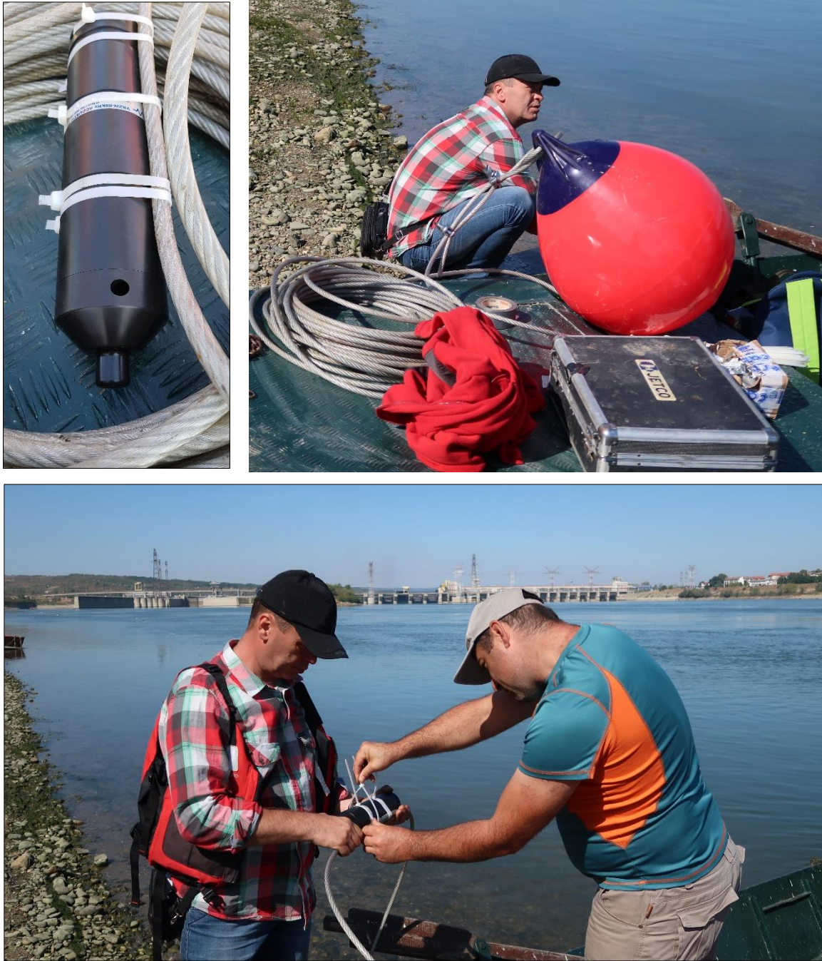
Figure 9. After release the fish were recorded by using stationary receivers, which automatically stored information on the date, time and identity of tagged fish when they were within the detection range of the receiver. For the tags with a depth sensor, the current swimming depth was also recorded. The upper left photo shows one of the receivers. Receivers were attached to wires, which were anchored to the bottom and held upright in the water column by floaters at the surface. Data were later downloaded to a computer. The study period in autumn 2019 lasted until the download of data from the receivers on 16 December 2019, and in spring 2021 until download of data on 16 June. Locations of receivers in the two study years are shown on the map in figure 11 . Photos: Eva B. Thorstad and Finn Økland.
