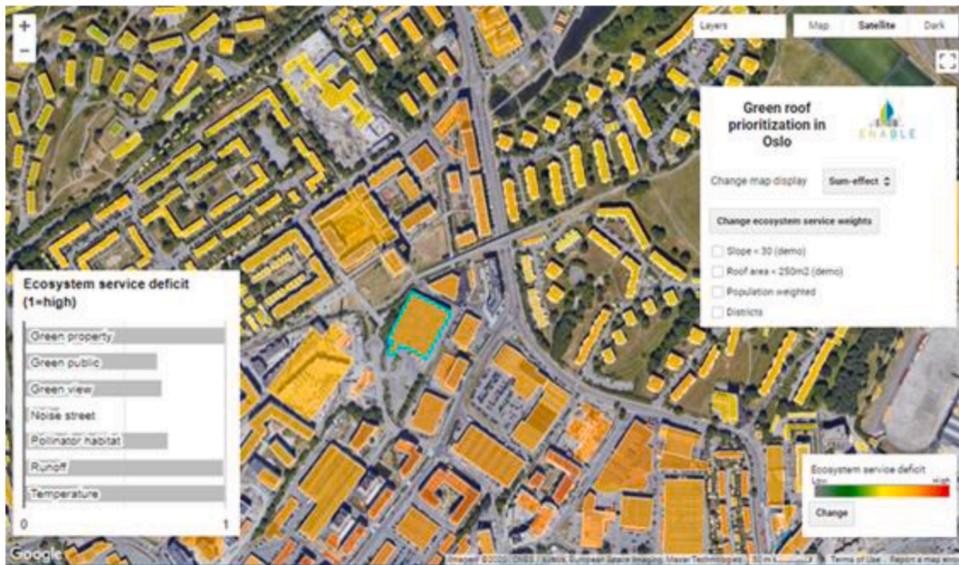
Fig. 6. Screenshot of the MCDA web application highlighting the ability to select individual roofs (blue border) and extract statistics of ecosystem service deficit scores.
