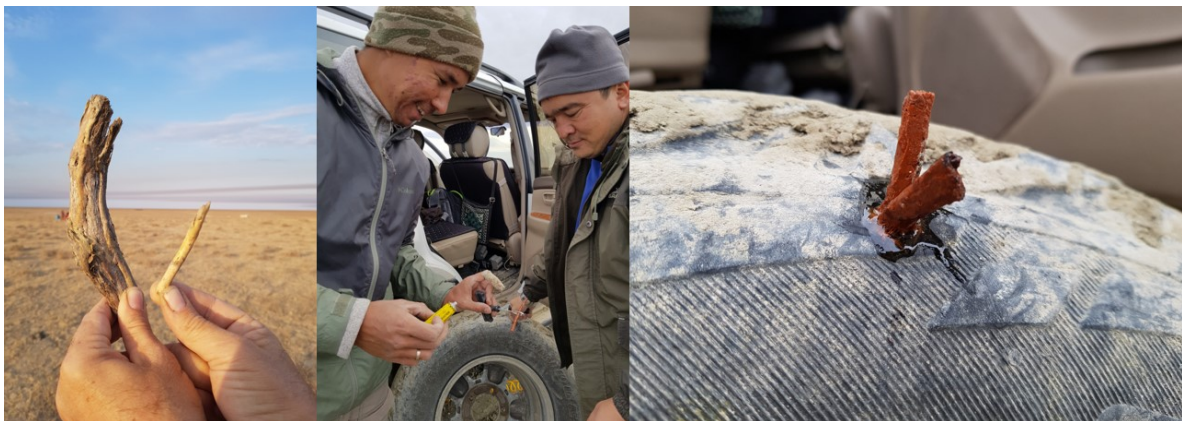
Fig. 28: Continual saxaul punctures eventually destroyed the tires to a point when driving was not safe anymore. Photos: P. Kaczensky
