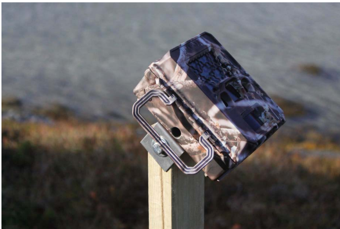
Figure 27. Reconyx high performance surveillance camera deployed to monitor the eagle owl behavioural responses on the new perching alternative on the pylon crossarm. Photo: Jan Ove Gjershaug.
