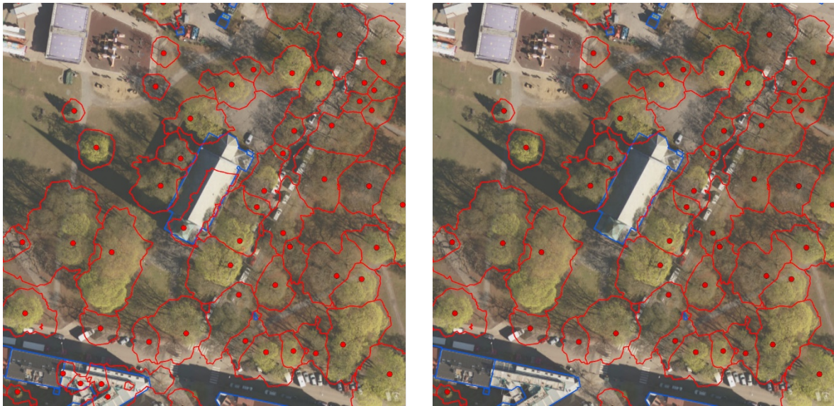
Figure 23: The image to the left displays the unmasked trees (in red) and the building mask (blue). The image to the right displays the trees (in red) remaining after filtering for interception with the building mask (blue).
