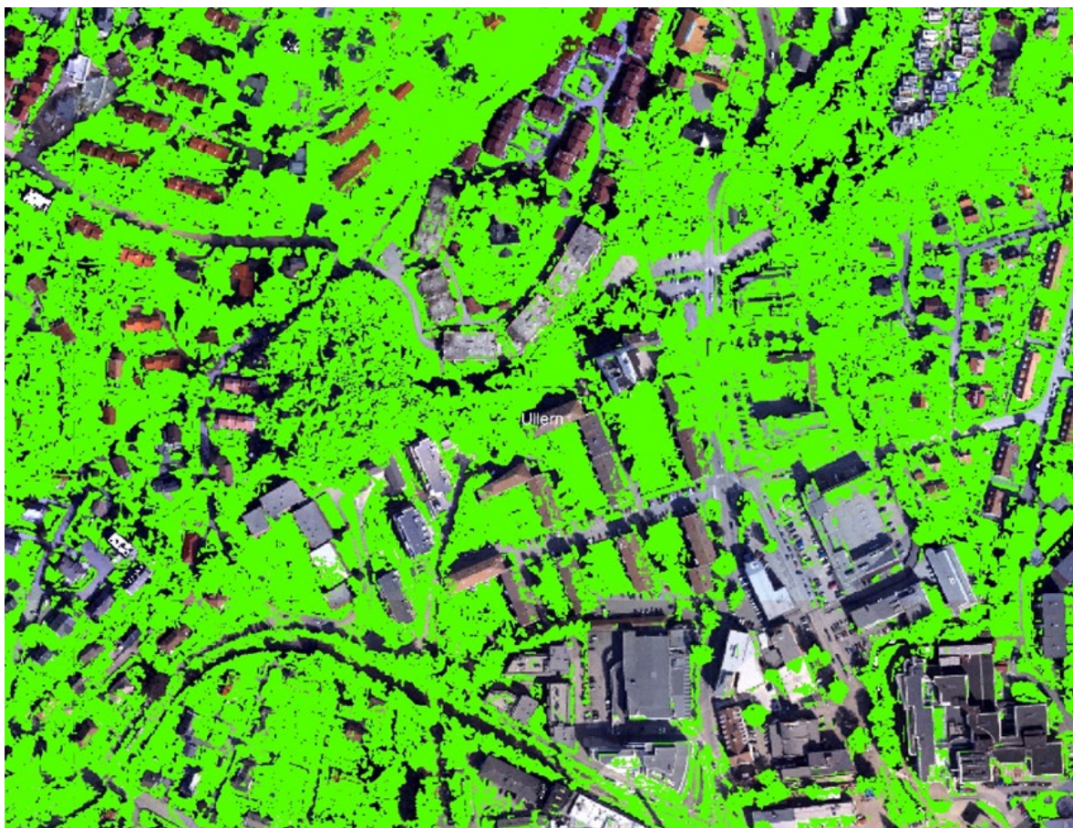
Figure 15: The Triangular Greenness Index (TGI) mask for the URBAN EEA field sample block 150 in the city district Ullem.
