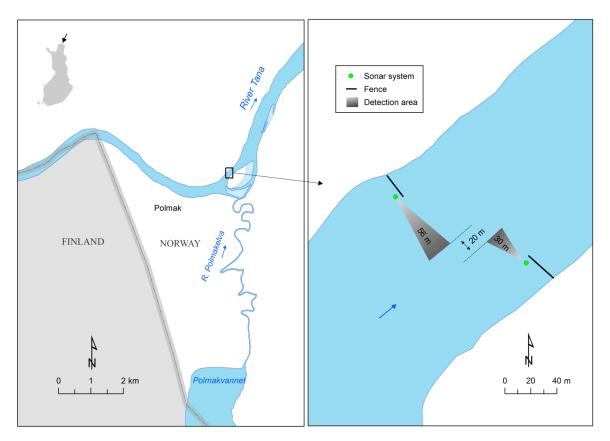
Figure 11. Map of the Tana/Teno main stem sonar counting site including the locations of the sonar units and guiding fences. The map also shows the c. 20 m wide unmonitored area.
