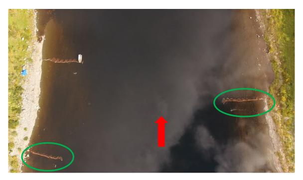
Figure 12. An aerial photo from the Tana/Teno main stem sonar counting site at Polmak. The sonar units within the green ovals were used in producing the salmon run estimate. Flow direction is indicated by the red arrow. Photo: Jari Lindeman (Luke).
