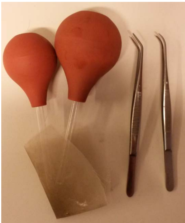
Figure 3. Picking equipment. Sucking organisms from the sample with a rubber bulb mounted on a 10 mm glass tube, and squirt them into a small net, allows for a much more effective sorting than forceps alone.
