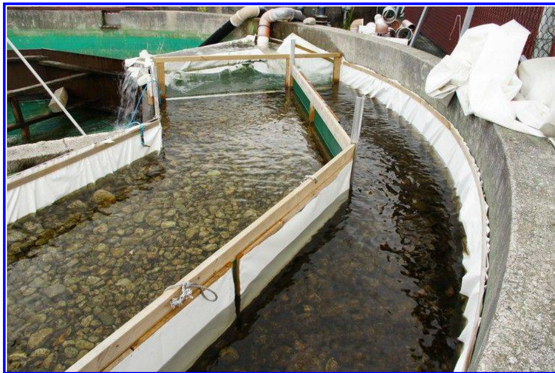
Fig. A6: Arena during fishing: The tarps are removed and the trap doors are lowered to separate the shallow from the deep area.
