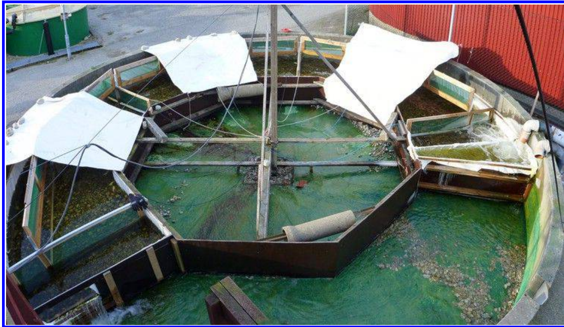
Fig. A4: One of the arenas used in the experiments. The water inlet is on the right side, the water outlet on the left. White tarps are providing shade and overhead protection. The photo depicts the 20 hour acclimatisation period when fish could swim freely around in the sections to choose their preferred habitat, i.e. the deep area close to the outer wall or the shallow area close to the inner wall. The mesh screens (“trap doors”) are therefore in the upper position, suspended over the water surface. The ropes that are used to activate the trap doors are leading to the centre of the whole construction, which is the place the operator will be standing when releasing them and thus ending the 20 hour acclimatisation period.
