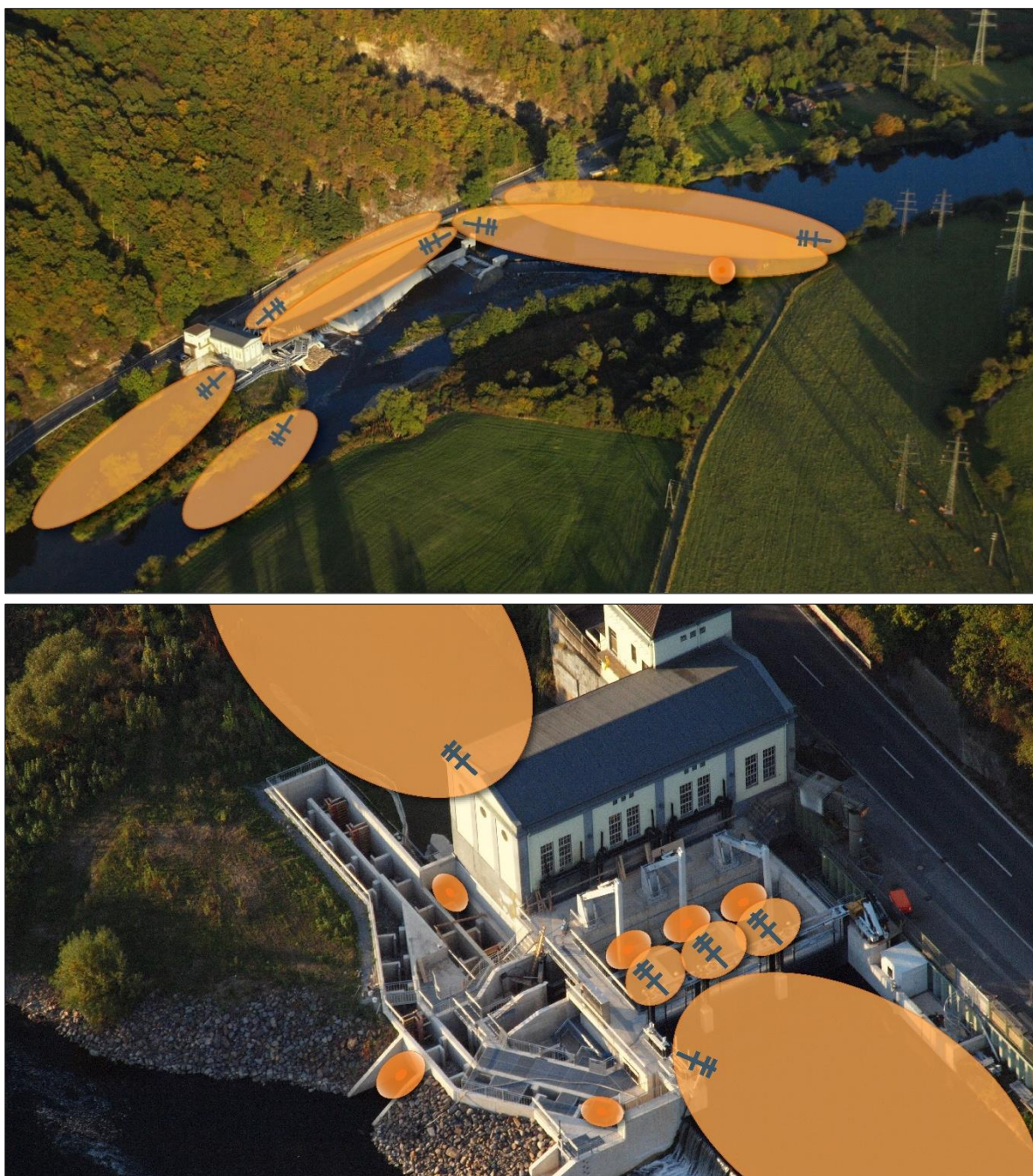
Figure 3.3. Overview of radio antennas and their approximate detection ranges used to record signals from radio tagged smolts at Unkelmühle power station. Upper panel: Overview of the power station area. Lower panel: Power station area in more detail. Detection ranges with antenna symbols indicate the use of aerial Yagi antennas, whereas ranges without antenna symbols indicate the use of underwater coaxial antennas Photos: Wikimedia Commons.
