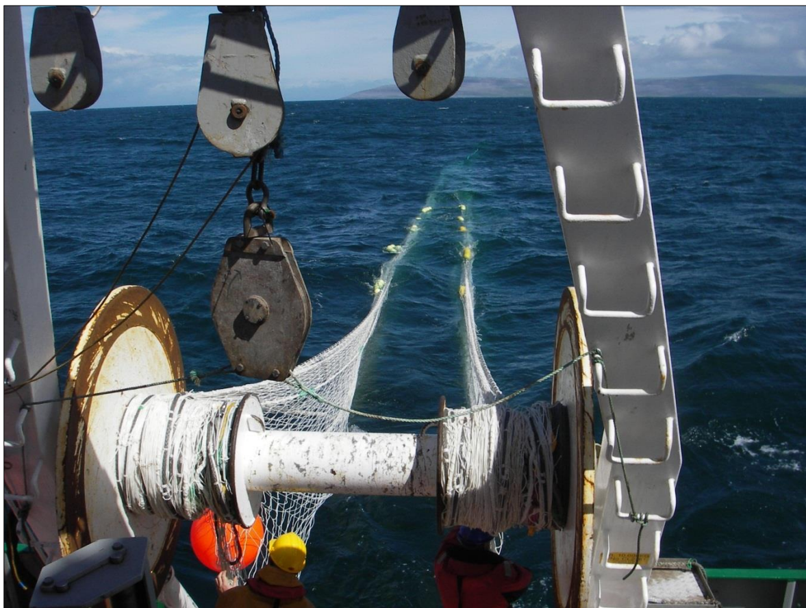
Deploying an ocean trawl net for Atlantic salmon post-smolts off the Irish coast. Photo: Patrick G. Gargan
