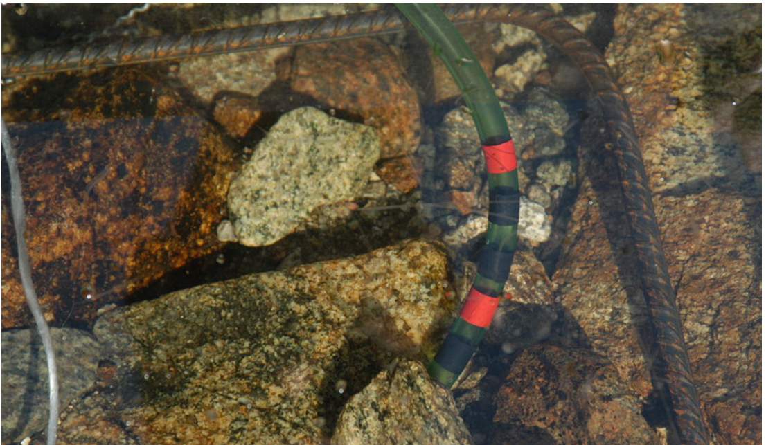
Figure 7. Measurement of sheltered habitat using a 13 mm-thick plastic hose inserted into interstitial spaces between rocks within the area of a 50 x 50 cm steel frame. Photo: Anders G. Finstad
