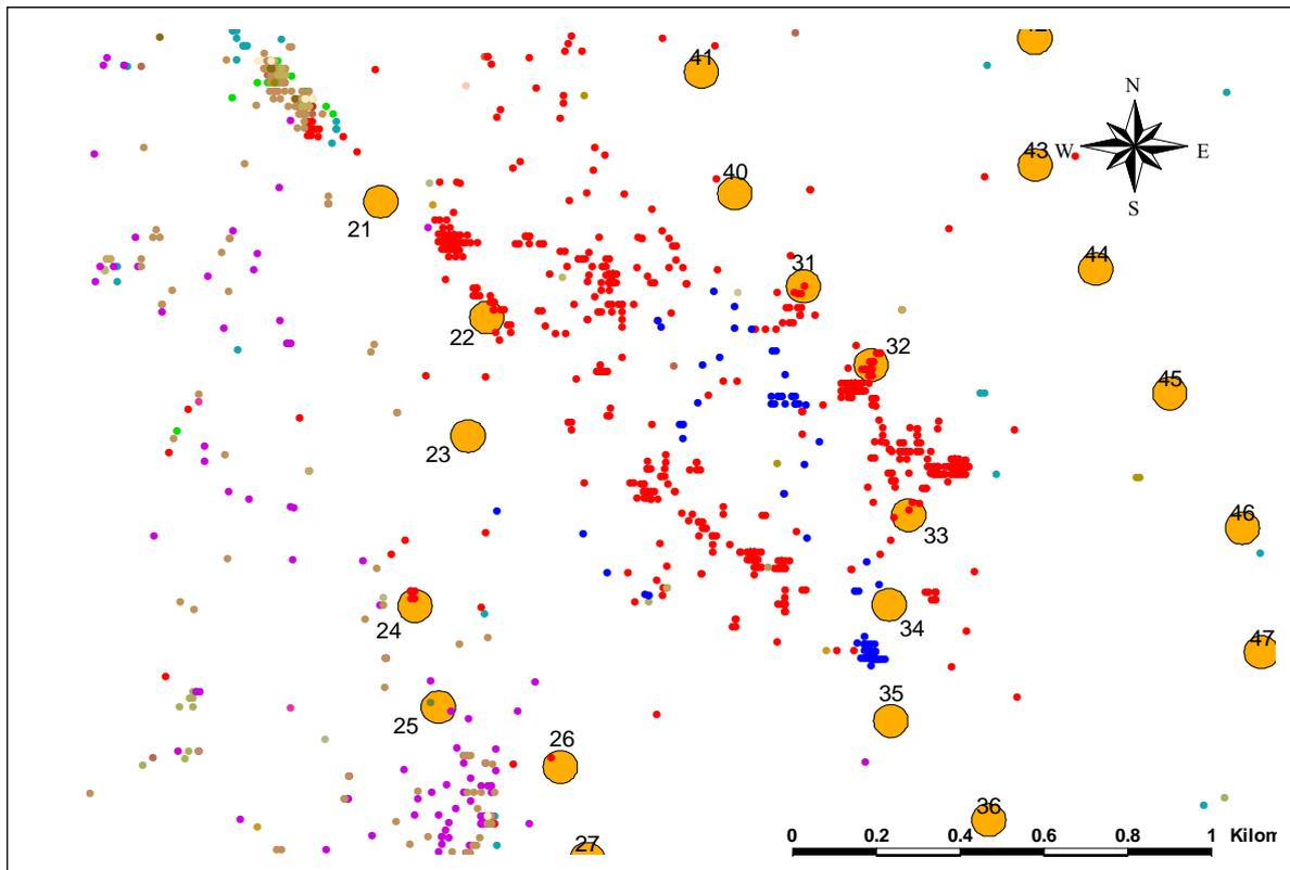
**Figure 16.** GPS positions of juvenile white-tailed eagles in the northwestern corner of Smøla Wind-Power Plant. Same colour indicates same bird. The rotor-swept zone of the wind turbines are shown as yellow circles (41 meter radius), and denoted by their number in the park. The GPS accuracy is 10-15m.
