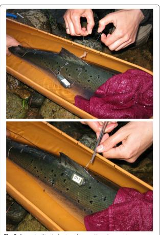
**Fig. 3** Example of typical external transmitter placement on a fusiform-bodied fish (Atlantic salmon, *Salmo salar*). This radio tag has a flattened section that lies close to the body surface and is held in place by stainless steel wires through the musculature. Note that these tags have conspicuous return information, which is not problematic for adult salmon, but could be an issue for smaller fish that may be susceptible to increased predation risk
